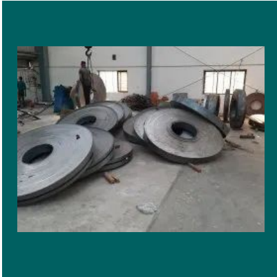
Hr Slit Coils
